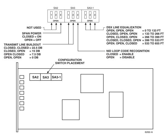
Figure 525-1. Version A RLX Configuration Switches
